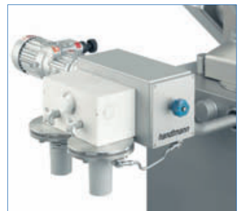
Meat ball device type 79-0. The meat ball device is connected directly to the outlet of the vacuum filler. The vacuum filler feeds the device continuously with evacuated product. The desired diameter of the meat balls is set on the forming device.
