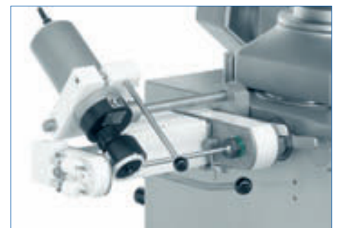
Casing spooling device type 78-6. Ideal for increasing capacity of sausage production in natural casings. Fast and gentle spooling onto the linking nozzle.
