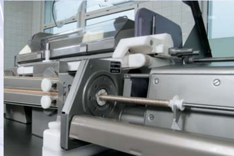
Linking unit with automatic casing changing. Quick and reliable feeding of peel-off and collagen slugs and gentle linking.
