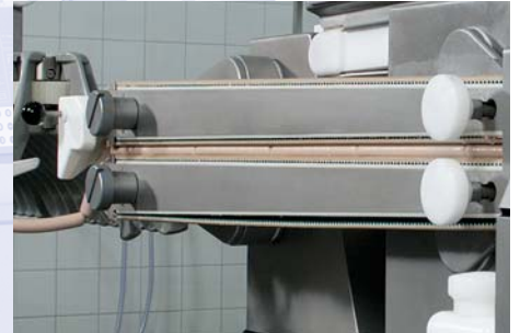
Equal lengths. The length unit guarantees equal sausage lengths with accurate portion weights.
