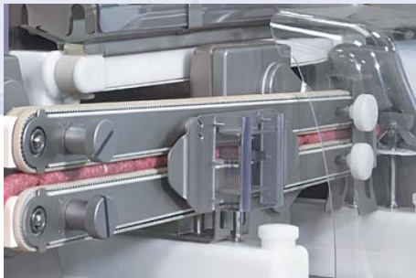
Voider and cutter. Reliable linking by the voider and precise separation of the portions by the cutting unit.
