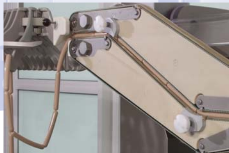
Reliable hanging. Gentle sausage transfer on hooks. Reliable and precise up to 3,000 portions per minute.
